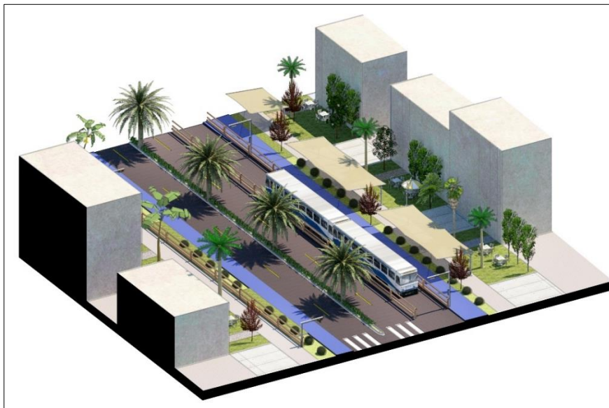
Image 11. Illustration representing green street guidelines. Natural shading, pedestrianism, utility corridors, public transport and use of soft permeable landscaping to enhance the user traffic experience.
